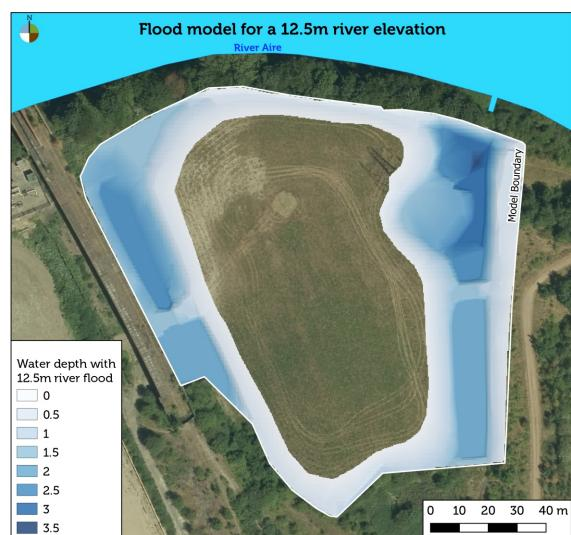
Challenge Three: To design the capping and surface water management system within a flood risk zone.
